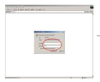
The Linksys router requires a User Name and Password in order to access the Configuration. (By default User Name is empty and Password is *"admin"*). Type this in and press 'OK'. The following 'Setup' screen will appear.
